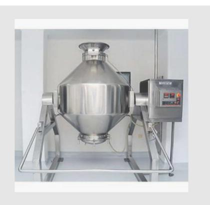
Equipment: Double Cone Blender. Application: Powder homogenizer.
