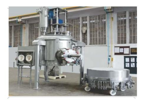
Equipment: Rapid Mixer Granulator (RMG). Application: FG Mixer and granules-making
